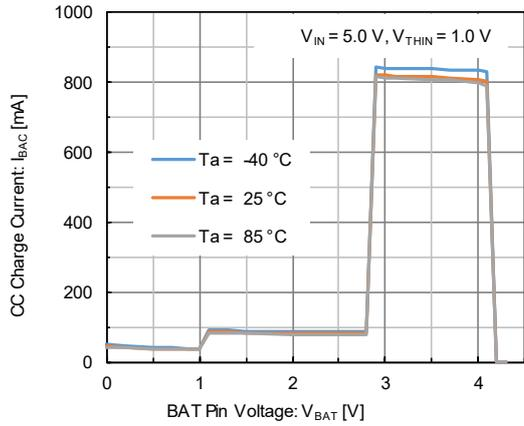
(13) CC Charge Current vs. BAT Pin Voltage
