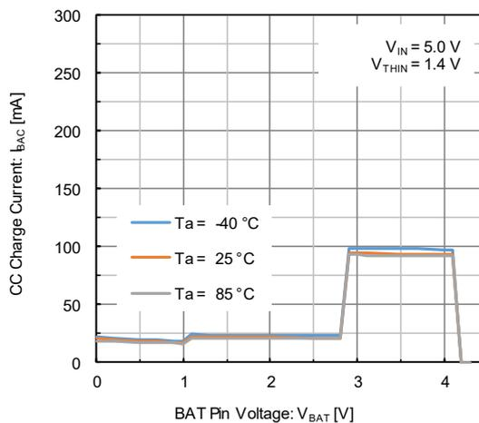
(10) CC Charge Current vs. BAT Pin Voltage
