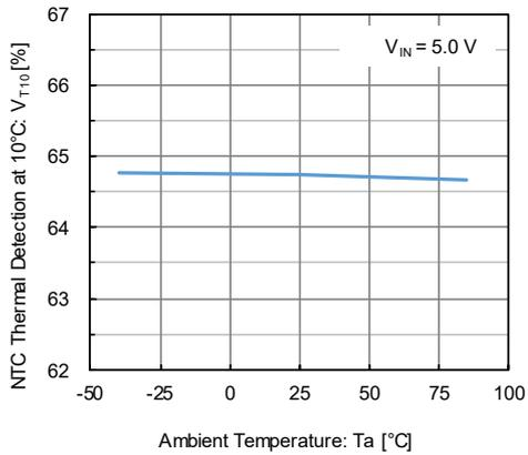
(37) Thermistor Detection Hysteresis at 10°C vs. Ambient Temperature
