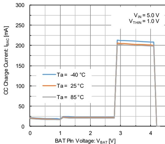
(9) CC Charge Current vs. BAT Pin Voltage
