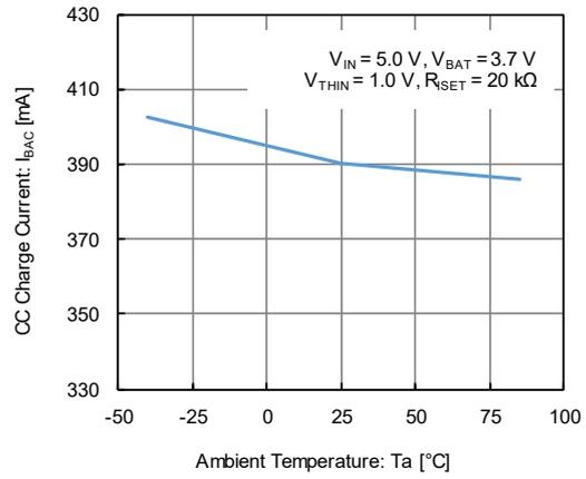
(3) CC Charge Current vs. Ambient Temperature (Cold Operation)
