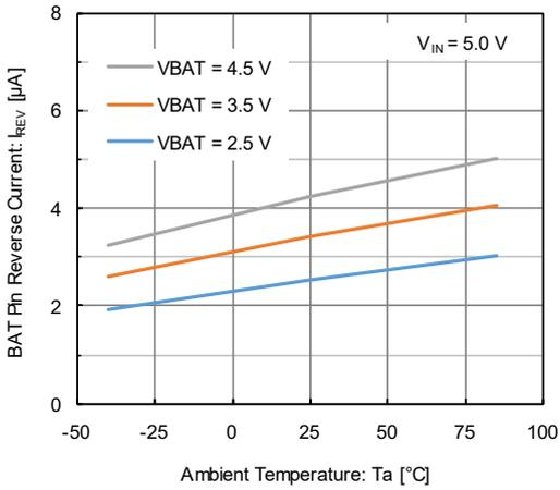
(27) BAT Pin Pull-down Current vs. Ambient Temperature
