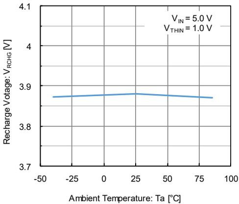
(29) Recharge Voltage vs. Ambient Temperature (Hot Operation)
