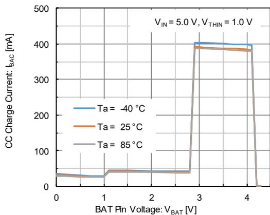
(11) CC Charge Current vs. BAT Pin Voltage
